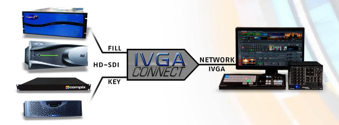
IVGA CONNECT™ EMPLOYS THE HOST GRAPHICS SYSTEMS HD-SDI FULL BANDWIDTH KEY AND FILL OUTPUTS, WHICH GUARANTEES THE HIGHEST QUALITY IVGA CONVERSION. IN ADDITION, SINCE IVGA CONNECT USES THE ACTUAL HD-SDI SYSTEM OUTPUT, ALL OF THE ASSETS ASSOCIATED WITH SCENE ARE AVAILABLE OVER IVGA.
